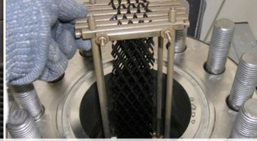
Thermo-oxidative ageing in a high pressure autoclave
