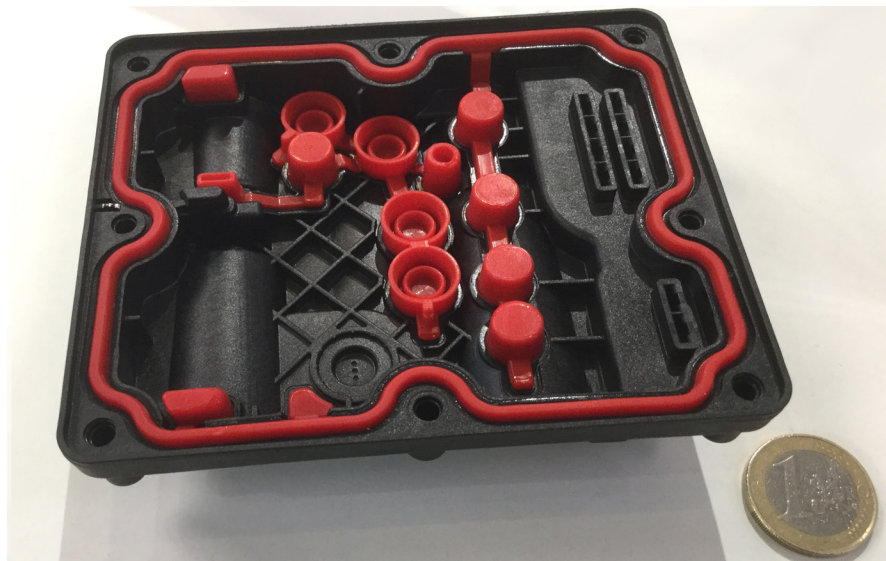
Two-component LSR/GF-PA molding displayed by KraussMaffei at the 2017 VDI Plastics in Automotive Engineering Congress.
